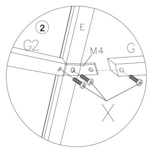
Affix solidifying bars to corner bar using iron angle (Part M4) and screws X as shown in diagram.
