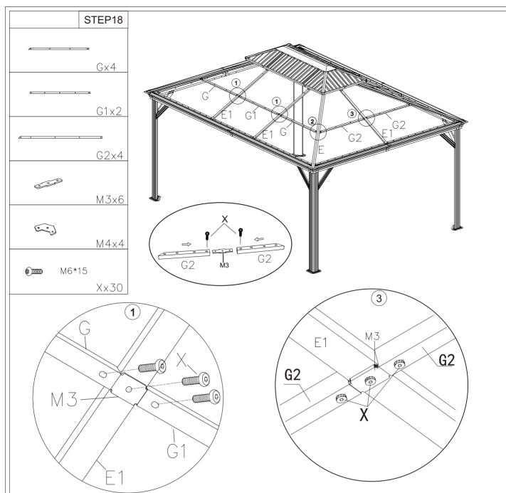
Affix solidifying bar (Part G,G1&G2) to roof bar or corner roof bar using iron angle (Part M3) and screws X as shown in diagram.
